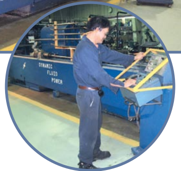
Large Industrial Honing Bench enables us to work materials up to 22" in diameter and 17' in length
