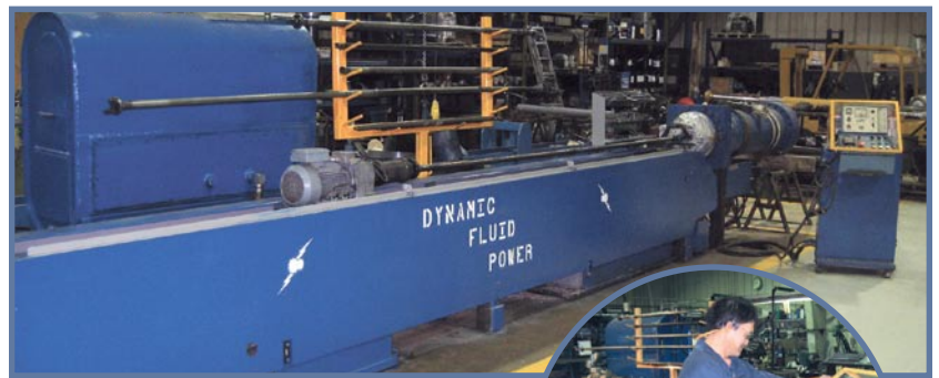
Large Industrial Honing Bench enables us to work materials up to 22" in diameter and 17' in length
